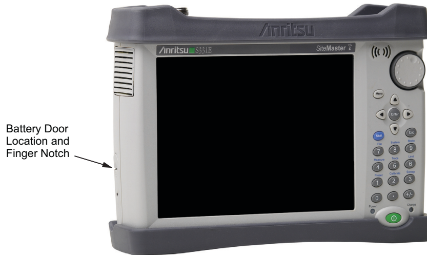
Figure 5-1. Battery Access Door Location and Finger Notch
