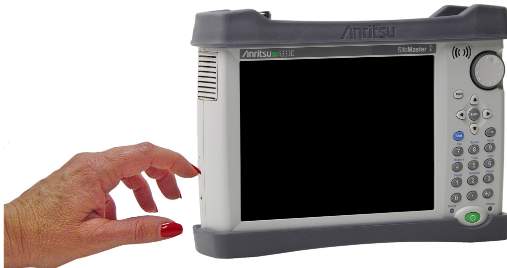
Figure 5-2. Opening the Battery Access Door
